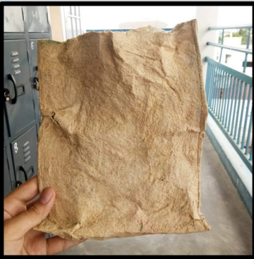
Final product of corn husk as efficient alternative plastic bag experiment
