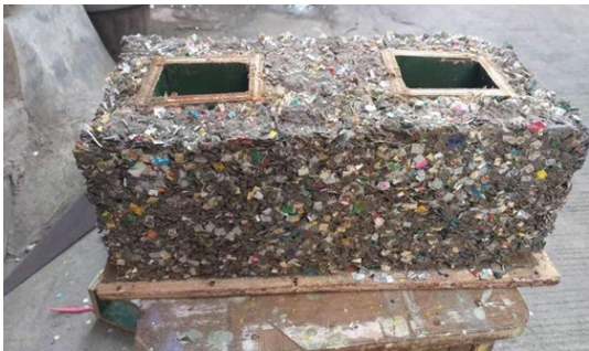
Final product of the Plastic Hollow Block experiment
